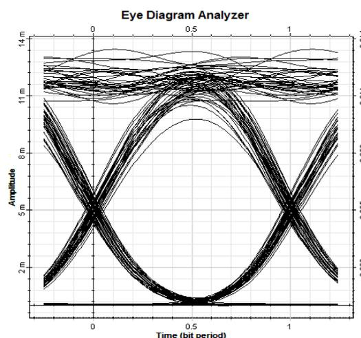
Fig. 11. (b) Eye diagram of the channel 8 with FBG as the dispersion compensation technique using NZDSF
