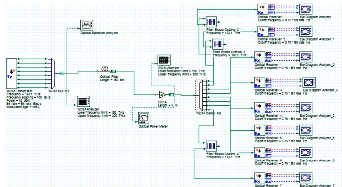
Fig. 6. DWDM Simulation model for the compensation technique with FBG
