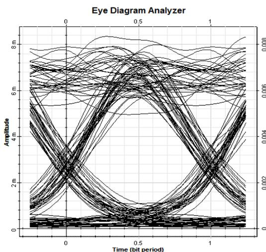
Fig. 8. (b) Eye diagram of the channel 8 with DCF as the dispersion compensation technique using NDSF
