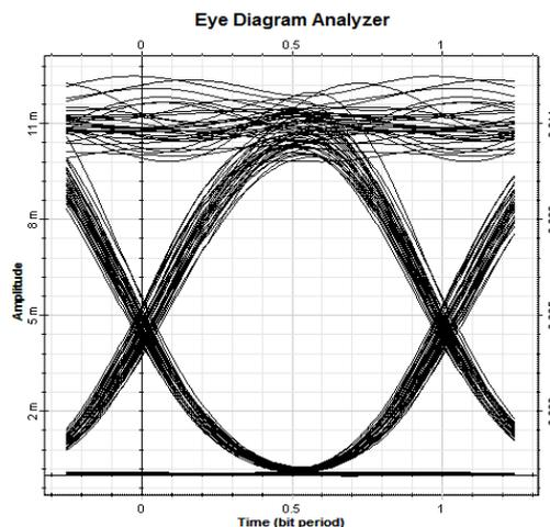
Fig. 11. (a) Eye diagram of the channel 1 with FBG as the dispersion compensation technique using NZDSF
