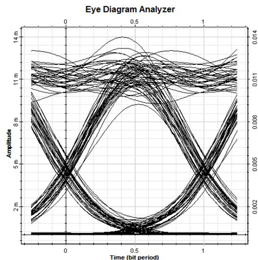
Fig. 9. (b) Eye diagram of the channel 8 with FBG as the dispersion compensation technique using NDSF
