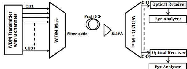
Fig. 3. Block diagram of DWDM compensation technique with DCF
