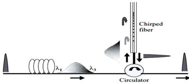
Fig. 2. A Chirped FBG with Circulator principle [8]
