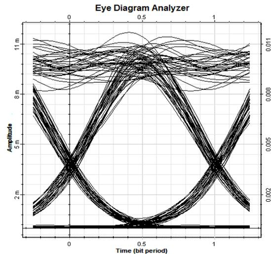
Fig. 9. (a) Eye diagram of the channel 1 with FBG as the dispersion compensation technique using NDSF
