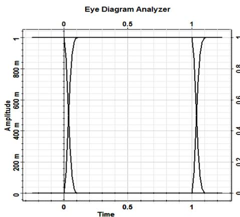
Fig. 7. (a) Eye diagram of the signal at the optical transmitter
