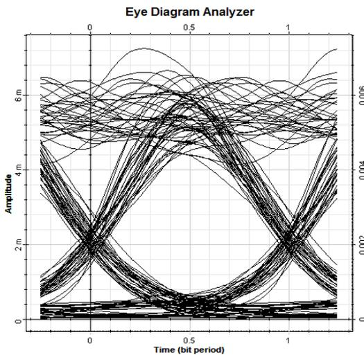
Fig. 8. (a) Eye diagram of the channel 1 with DCF as the dispersion compensation technique using NDSF
