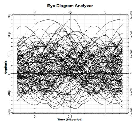
Fig. 7. (b) Eye diagram of the signal at the optical receiver without dispersion compensation
