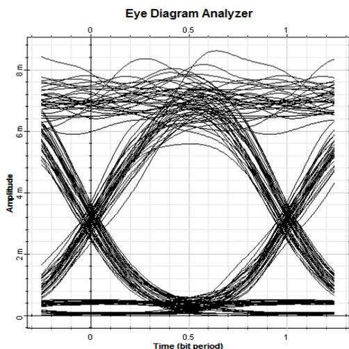
Fig. 10. (a) Eye diagram of the channel 1 with DCF as the dispersion compensation technique using NZDSF
