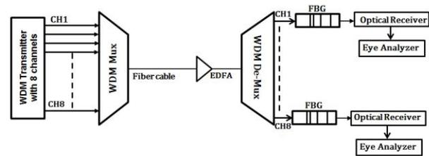
Fig. 4. Block diagram of DWDM compensation technique with FBG
