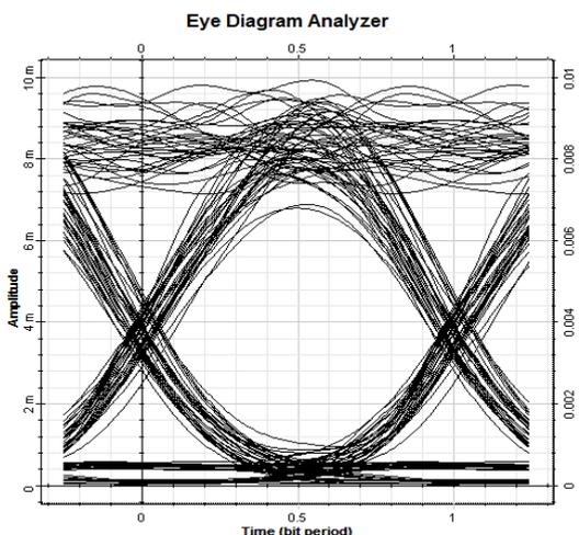
Fig. 10. (b) Eye diagram of the channel 8 with DCF as the dispersion compensation technique using NZDSF
