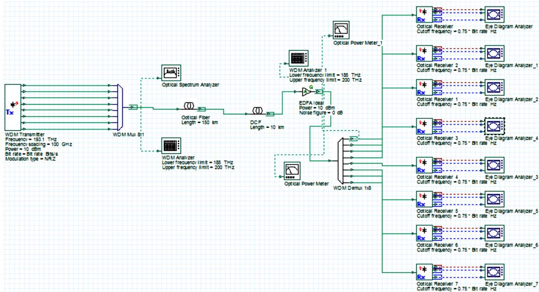
Fig. 5. DWDM Simulation model for the compensation technique with DCF
